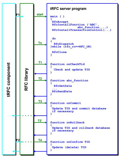
The tRFC component, the RFC library and the tRFC server communicate with each other in two phases:
