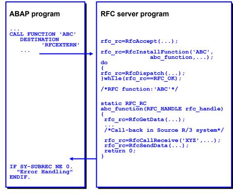
Function module 'XYZ' is any RFC-supported function module in this source R/3 System.
