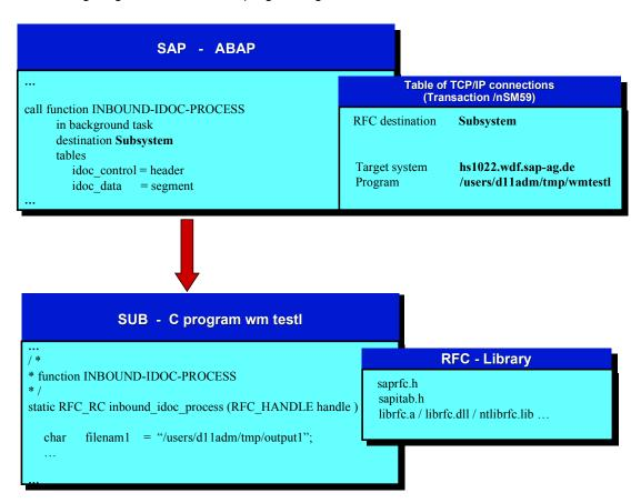
You transmit IDocs from the R/3 System by calling one of the two following functions modules with a destination:
