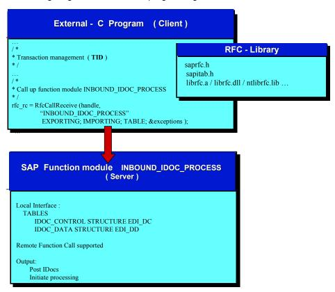
The calling, external program uses the following functions of the *RFC Software Development Kit* (RFC-SDK):
